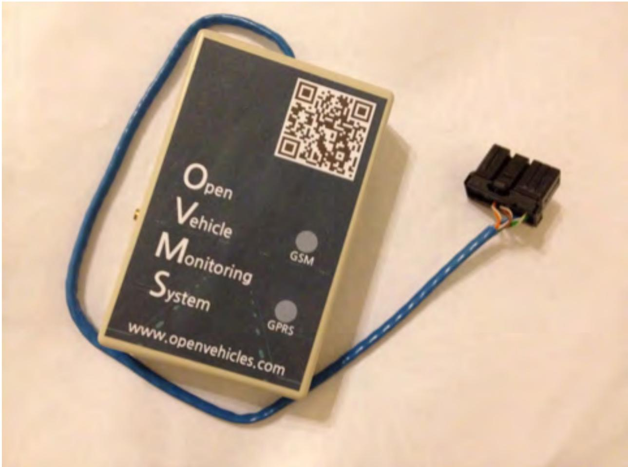
The OVMS module contains a low-power micro-controller control board and a GSM cellular modem. It plugs into the car's diagnostics port (from where it receives power and listens to the car's internal communications), and provides monitoring and control functions via either SMS messages or smartphone apps (over the Internet).
