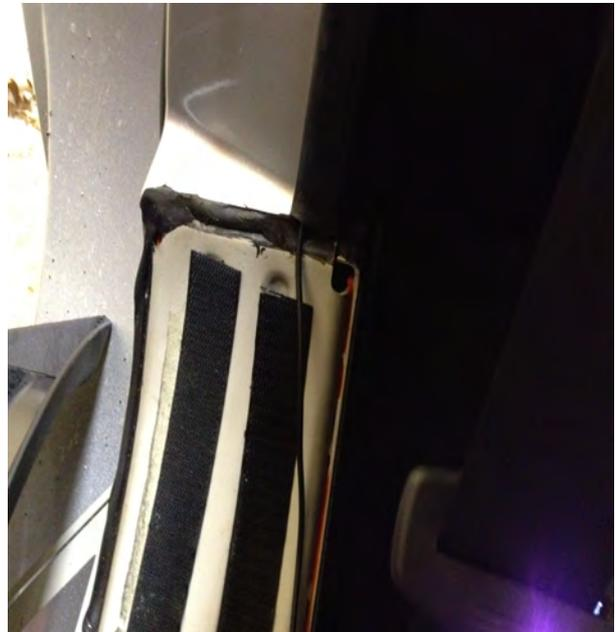
The antenna can either be placed on the plastic beside the door near the passenger's head, or further back in the rear window of the car.
