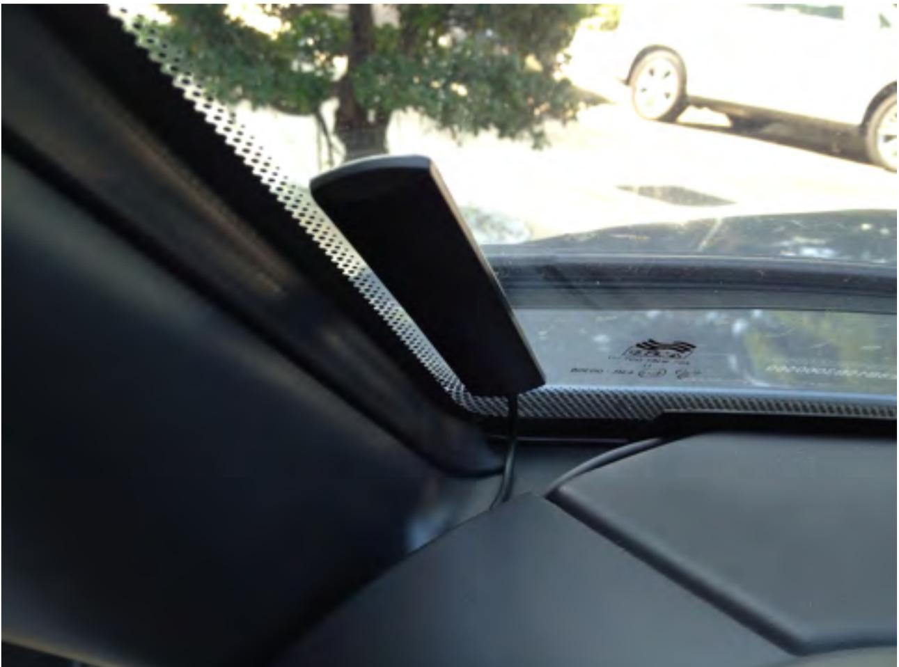
*Example antenna placement in a right-hand-drive car (left-hand-side passenger)*
